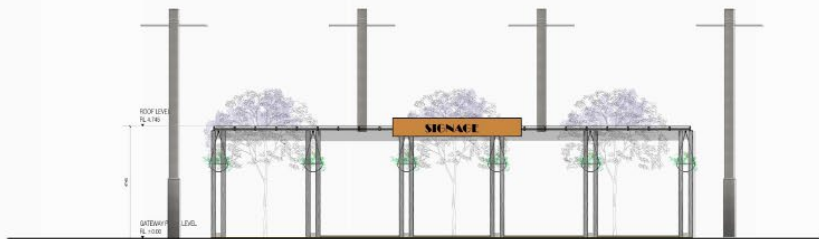
1.1 EASTERN PAVILION WEST ELEVATION SCALE: 1:100 @ A1
